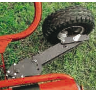
Changing from transport to work position
