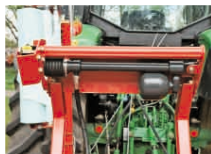
The hydraulic cutter gives a clean and secure cut.
