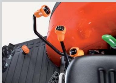
The gearbox ratios can be compounded by a mechanical underdrive giving a total of 20+10 speeds, with the further option of a creeper box for a total of 30+15 speeds.
