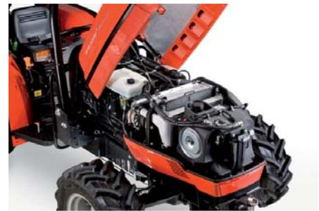
Another unique feature is the exclusive SDF fuel injection system, which uses an individual injection pump for each cylinder and is significantly more advanced than systems using rotary pumps. The SDF system guarantees a particularly high operating pressure (1400 bar) and instantaneous injection, which is governed by a load-responsive
