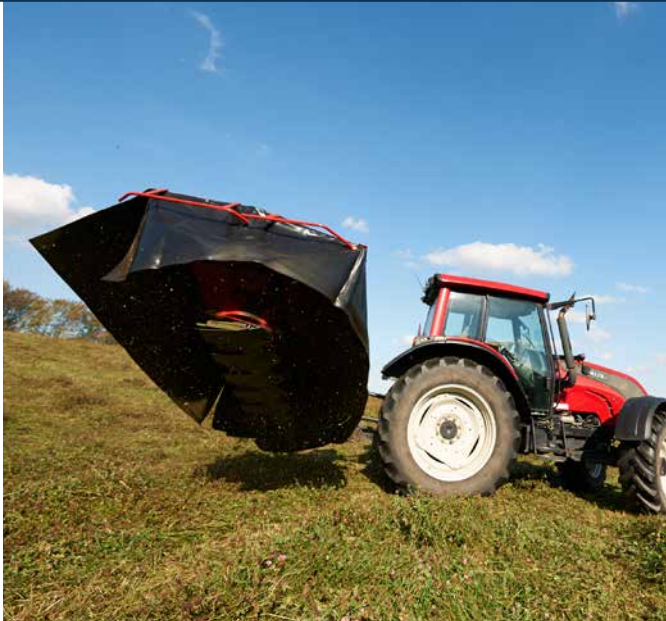
Lifting on headlands via a hydraulic cylinder.
