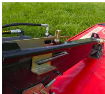
Any ground-unevenness are absorbed by the suspension.
