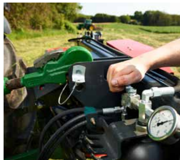
Hydraulic setting of ground pressure (EXTRA 432H and 436H).
