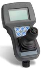
Portus joystick with all functions integrated.
