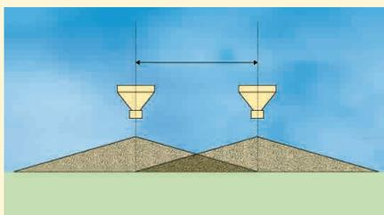
The cone shaped spreading pattern reaches from tractor wheel track to tractor wheel track giving total overlap of the spreading surface
