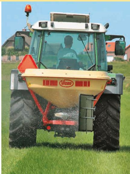
Border spreading with the border spreading plate
