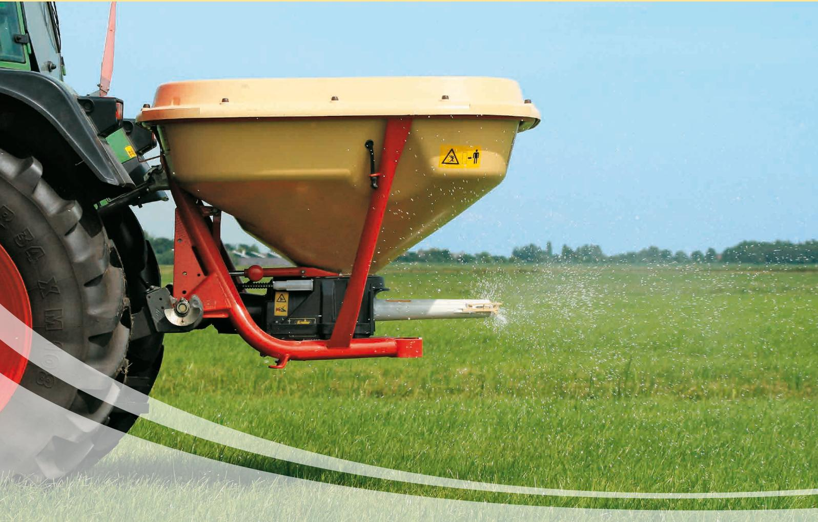
**More than one million machines sold prove that the Vicon pendulum seeder/spreader is the first choice wherever the demand is for maximum accuracy in fertiliser application. Spreading quality and ease of operation of this unique machine are unequalled - now as in the past. The pendulum movement of the spout ensures that the application rate is always identical on both sides. This results in an excellent overlap.**
