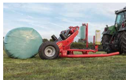
Low design of the machine ensures fast and gentle unloading of the bale.
