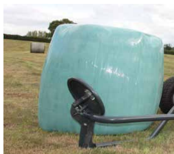
The Vicon BW2850 can be fitted with a bale on end kit.
