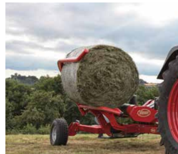
Hydraulically operated loading arm, and a low loading height, provides fast transfer of bale from arm to turntable.
