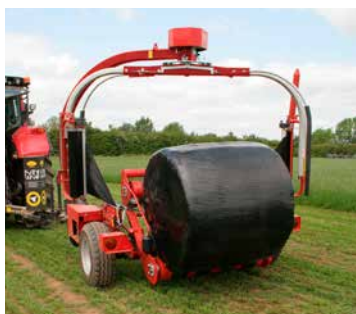
Fast and gentle unloading of bales with no need for a drop mat.
