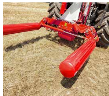
Easy and gentle self-loading of the bales – the bale is gently lifted by the rollers.
