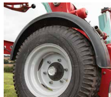
Mud guards reduce mud and dirt building up on the pre-stretcher and film rolls when operating in soft ground field and during transport.
