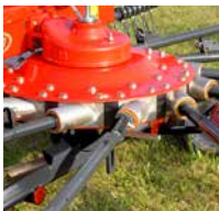
Tine arms can be easily removed.
