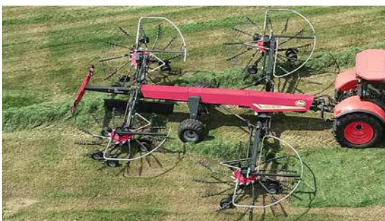
Vicon An dex 1304 Pro Individual lifting feature of all four rotors.
