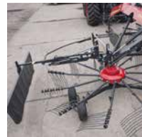
Automatic fold-able swath board with parking stand.
