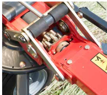
Vicon HexaLink finger clutch permits the rotors to fold 180° for transport.
