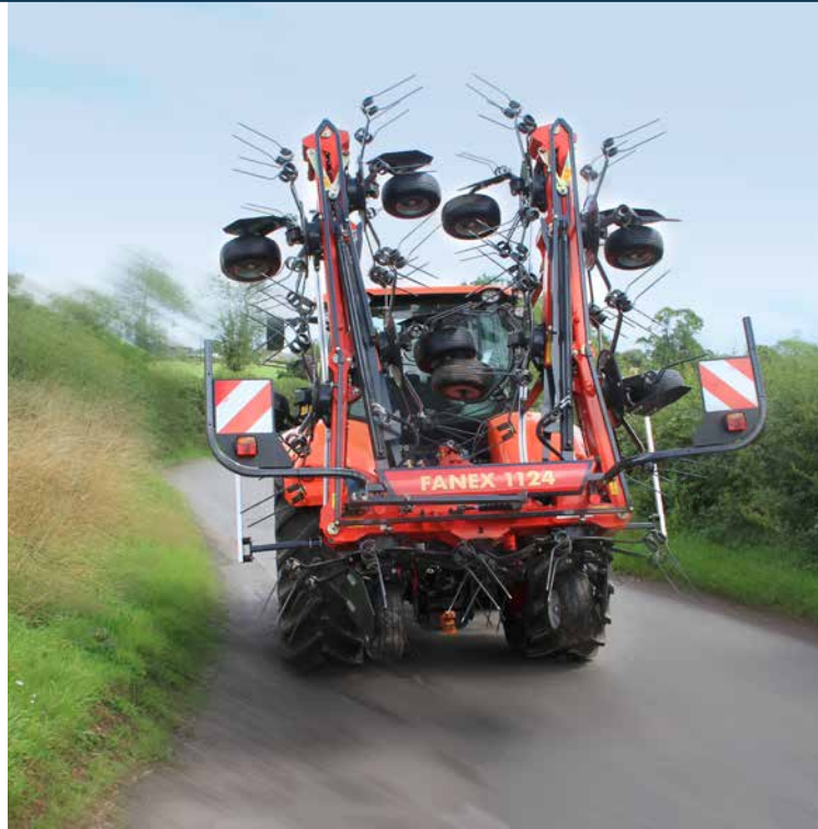
Compact transport dimensions of Fanex 1124 – storage height is only 3.80m.
