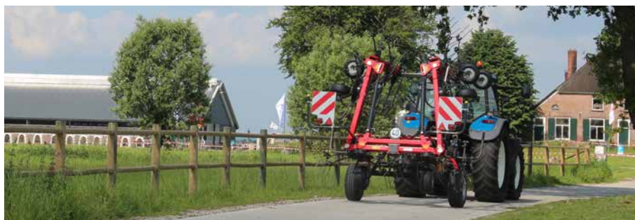
During transport both tedders have a height of only 3.35m.
