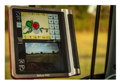
An 'IsoMatch Eye' rear view camera combined with the optional large screen Tellus Pro terminal allows the operator to keep a check on the wrapping process and safe bale discharge.
