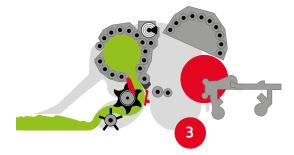
The tailgate opens and the completed bale rolls directly on to the wrapper by gravity.
