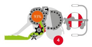
The wrapper is raised to its working position and wrapping commences.
