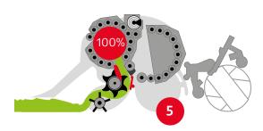
Crop flow continues to fill the pre-chamber until the preset density is reached.
