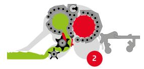
When the bale is fully formed, the crop flow, is diverted to pre-chamber, while net is applied to the completed bale.
