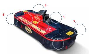
possible to the tractor, adding to stable and smooth running of the tractor, when going up and down steep slopes. The suspension concept allows a transverse adaptation of 28°, giving the mower outstanding flexibility.
