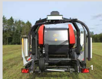
Once the net is applied to the bale the wrapping table moves forward under the tailgate of the baler.
