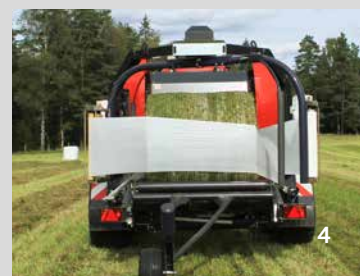
The wrapping table moves rapidly to the pre-stretchers and wrapping starts instantly.
