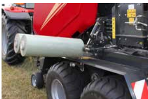
Stretch film cassette with hydraulic operation for maximum operator convenience.
