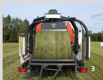
As soon as the bale is transferred away from the baler, the tailgate automatically closes, and baling can resume.
