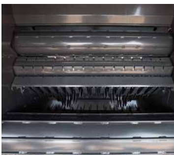
The bale chamber concept consists of five rollers at the front...
