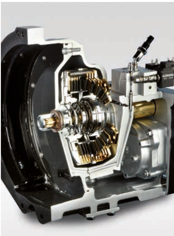
Power shuttle section with Stop&Go system
