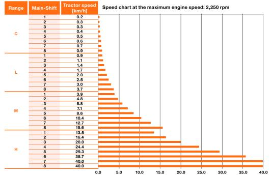
H7: 2,060 rpm H8: 1,689 rpm
