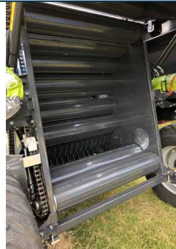
Lower main bale chamber with twin support rollers.
