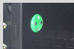
Moisture sensors located inside bale chamber.
