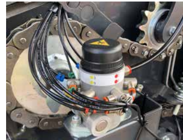
Automatic chain lubrication with individually adjustable outlets.
