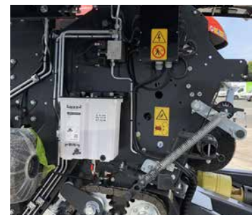
Rigid steel pipes for hydraulic circuits.
