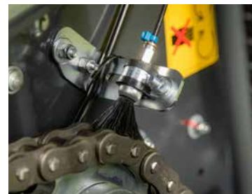
Automatic chain lubrication is standard on FixBale 500.
