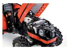
Another unique feature is the exclusive SDF fuel injection system, which uses an individual injection pump for each cylinder and is significantly more advanced than systems using rotary pumps. The SDF system guarantees a particularly high operating pressure (1400 bar) and instantaneous injection, which is governed by a load-responsive
